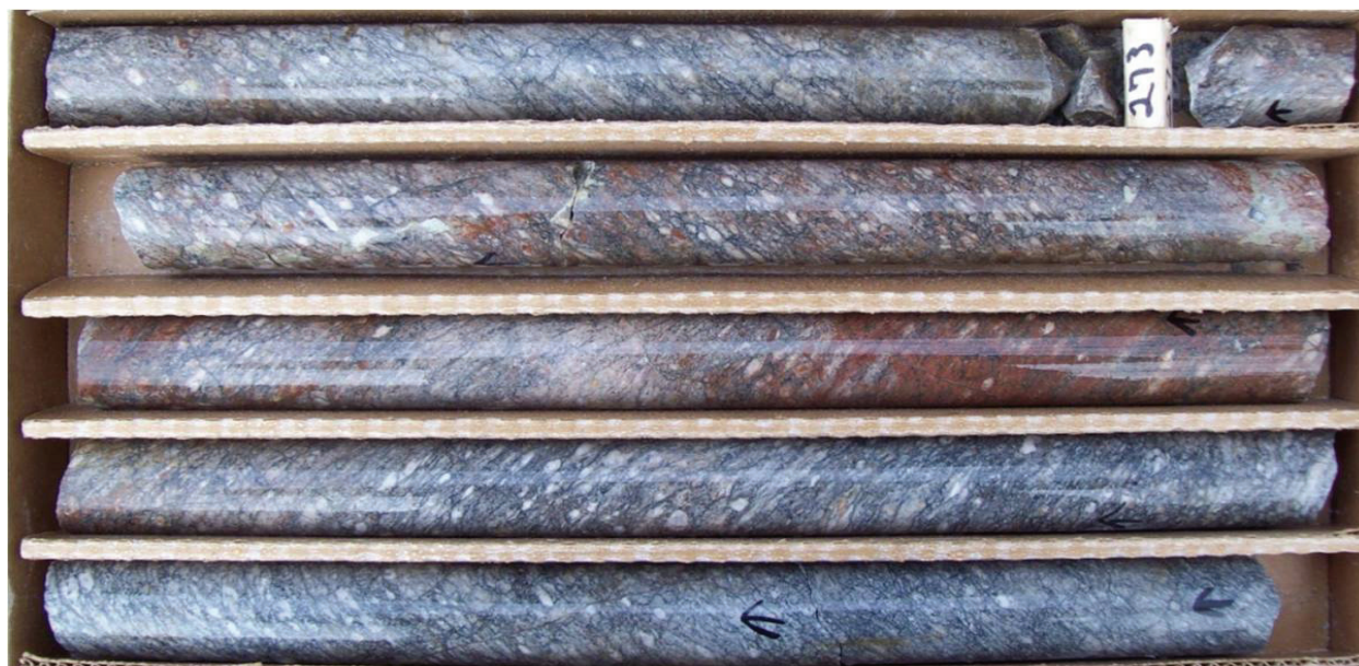
FIGURE 3.15 Drill core from the Leatherwood Granite showing highly sheared and mineralized granite. The average U_3O_8 percentage in this 10-foot core section is 0.679%. SOURCE: Wales (2010 49 ).
