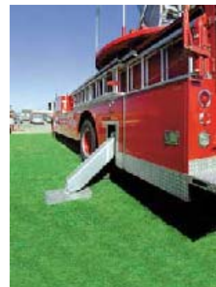
Outriggers used to stabilize fire trucks can extend the effective width of the vehicle by several feet on each side.
